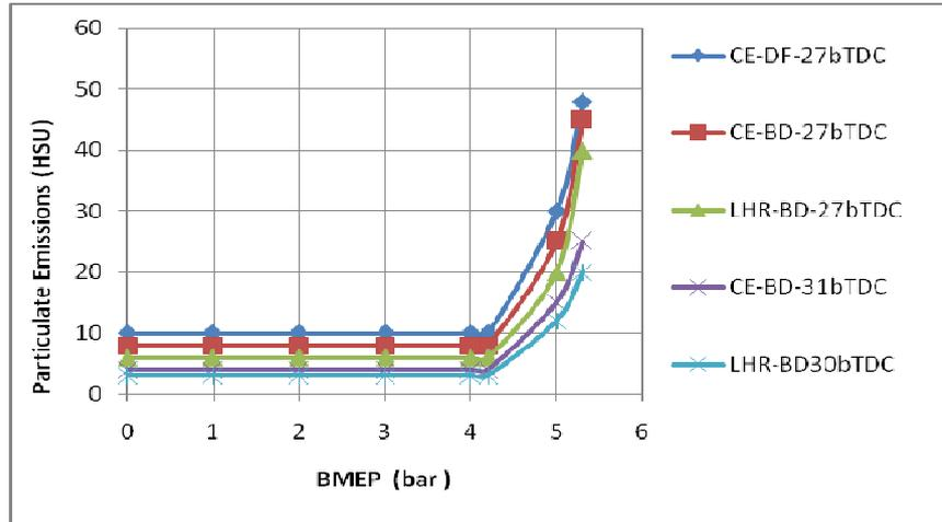
**Figure 4: Variation of Particulate Emissions in Hartridge Smoke Unit (HSU) with Brake Mean Effective Pressure (BMEP) in Conventional Engine (CE) and Engine with LHR Combustion Chamber at Recommended Injection Timing and Optimum Injection Timing and at an Injector Opening Pressure of 190 Bar with Biodiesel (BD)**
